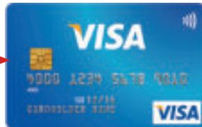
**Chip Antenna** for contactless cards, the interface can be an antenna embedded into the back of the card and connected to the chip. A contactless transaction works at terminals through the radio frequency wave between the card and the terminal.
